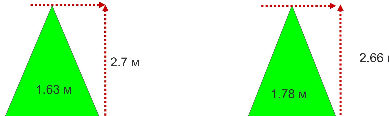
$$\frac{2.7 \text{ м} \times 1.63 \text{ м} \times 10'000 \text{ м}^2}{5.0 \text{ м}} = 8'800 \text{ м}^3 / \text{га}$$
